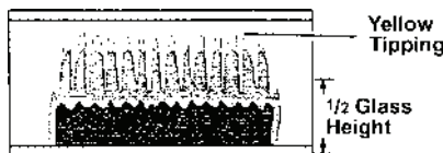
Figure 24 - Incorrect Burner Flame Pattern
