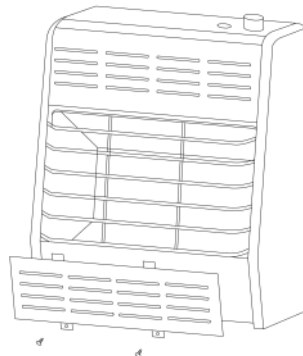
Figure 7 - Removing Lower Front Panel Of Heater
